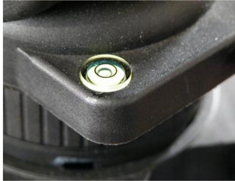
*Bubble level as part of the tripod head*
